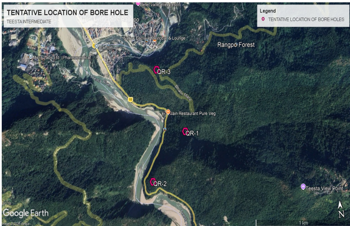
Figure III: Proposed Bore Hole Location
