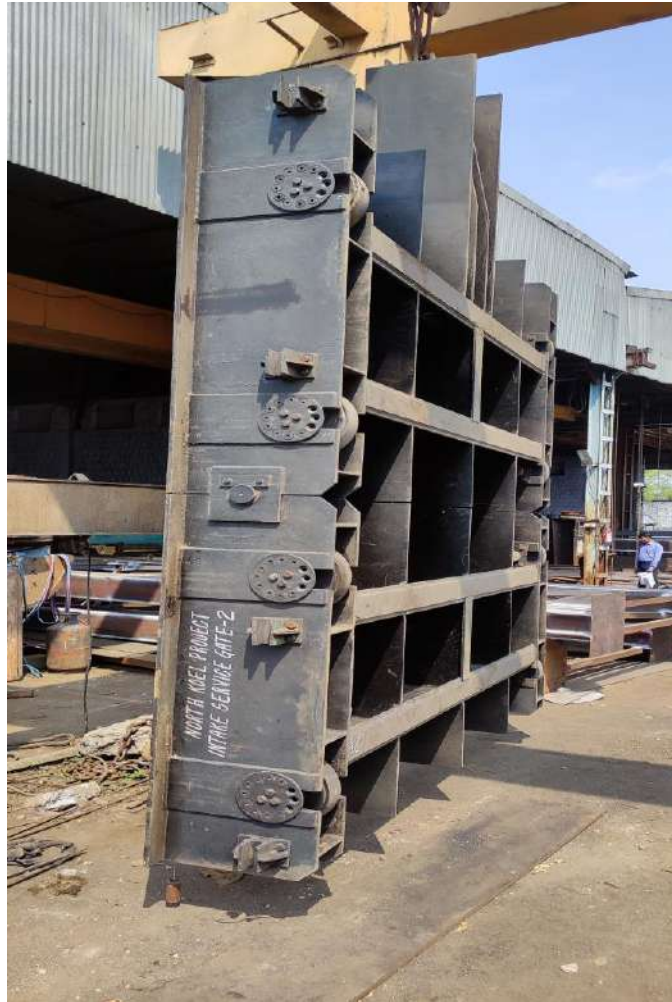
(A) Intake Service Gate (2.4 m x 3.066 m)
