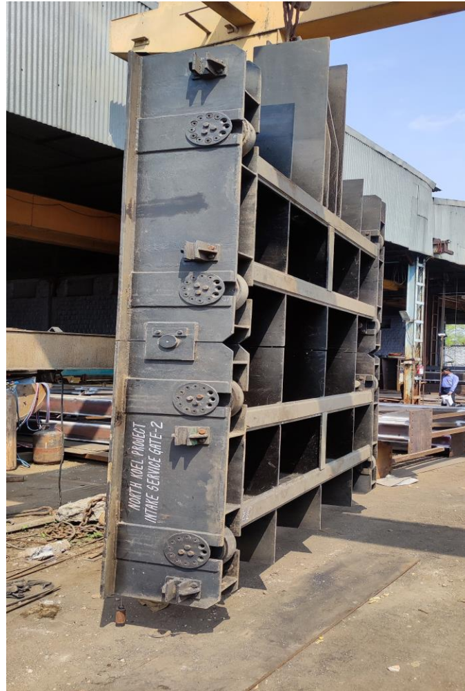
(A) Intake Service Gate (2.4 m x 3.066 m)
