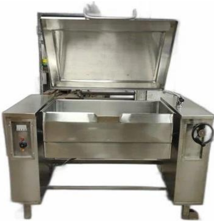
SS TILTING TYPE BOILING PAN OF 200 LTR
