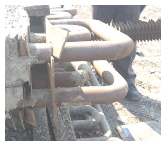
Deposition on Economizer Tubes
