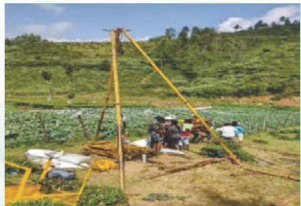
Conducting Goodman Jack test in drill hole at Right bank of River
