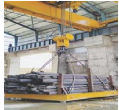
Ph-I Eot Crane (Overload Test)
