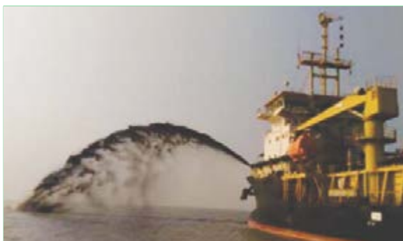
Dredging by Rain bowing method
