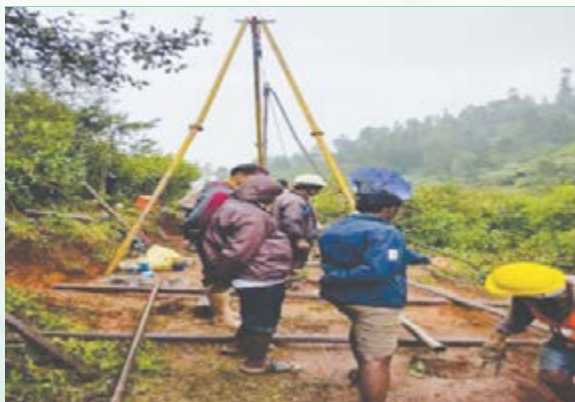
Conducting Goodman Jack test in drill hole at left bank of Sillahalla river at upper dam site
